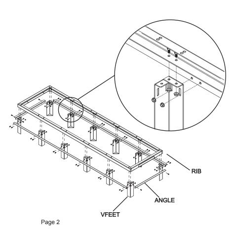
4) Mount the rack to the RIB: Using the supplied hardware bolt the rack to the RIB. Gang all of the racks mounted to the RIB using the following:
